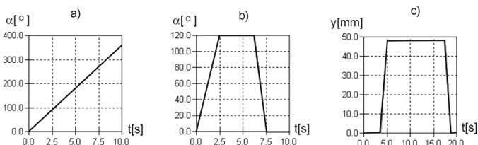
Fig. 6: Graphs presenting the work of the following drivers: a) main, b) correcting with a rotatable module, c) correcting with a movable support.
