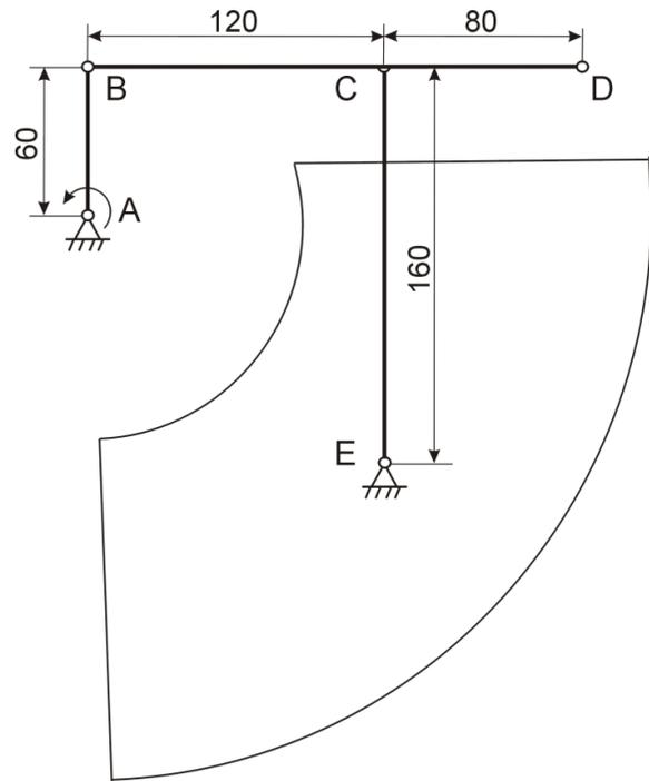
Fig. 1: The scheme of articulated quadrilateral used for tests.
