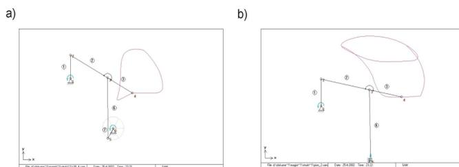
Fig. 5: Resulting trajectories implemented by mechanisms with an additional correcting drive.
