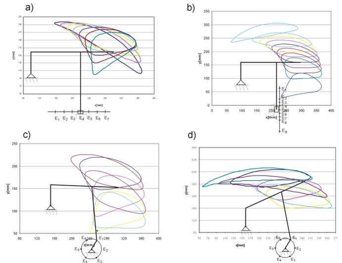
Fig. 2: Determined trajectories with the position change of E support as follows: a) horizontally b) vertically c) in a tangent circle below the support d) in a tangent circle below the support.
